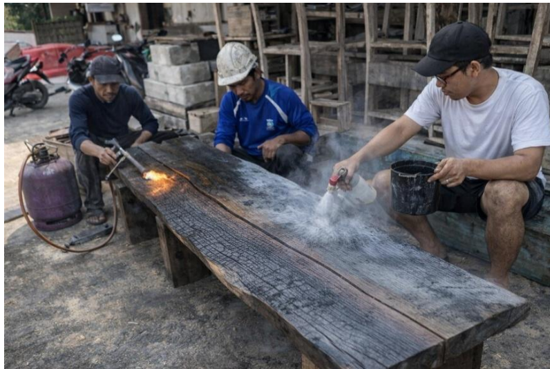
Figure 4. Antique Effect Produced through Controlled Burning
