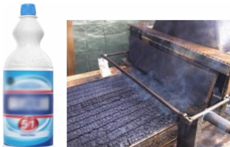
Figure 2. Carbonized Wood Surface after Controlled Burning
